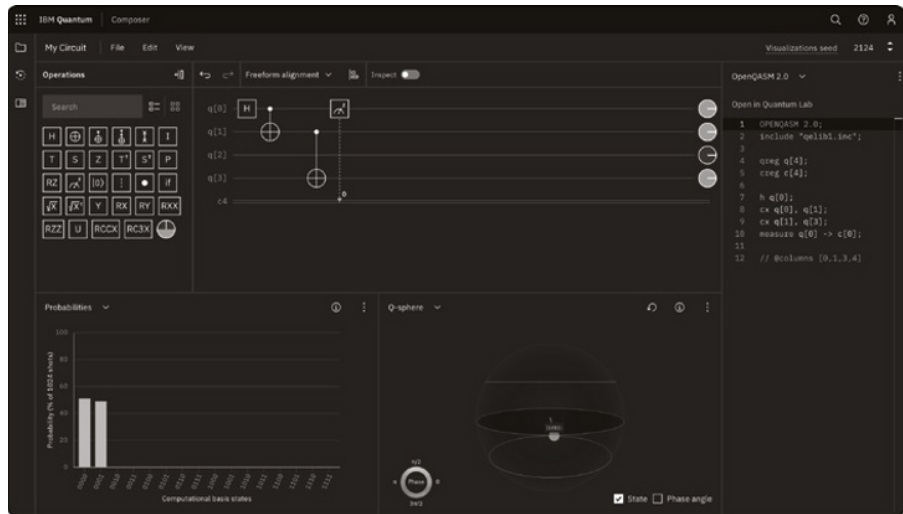
FIGURE 15-5: The IBM Quantum Composer is a no-code processing tool that emits Python code.
