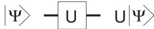
Fig 1.2 A circuit diagram representing the action on n Qbits of the n -Qbit gate \mathbf{U} . Initially the Qbits are described by the input state |\Psi\rangle on the left. The thick line (bar) represents the subsequent history of the Qbits. After emerging from the box representing \mathbf{U} , the Qbits are described on the right by the final state \mathbf{U}|\Psi\rangle .
