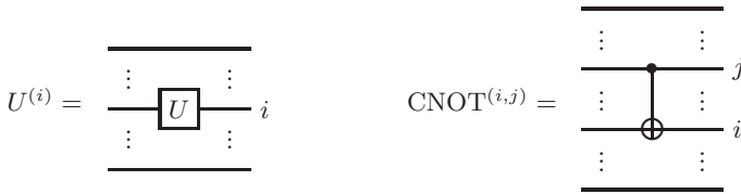
Fig. 4.1. Elementary quantum gates
