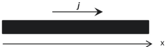
Fig. 1.14 Current in 1D wire. In the 1D case current I is simply proportional to j
