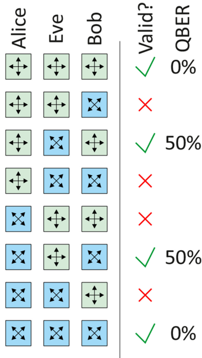
Figure 5.15. QBER caused by a man-in-the-middle attack.
