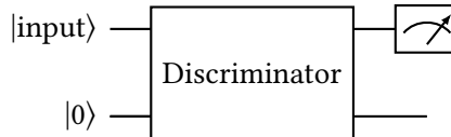
(c) Discriminator circuit, tasked with deciding whether the state |\text{input}\rangle is the state |\psi_1\rangle or the output of the generator.
