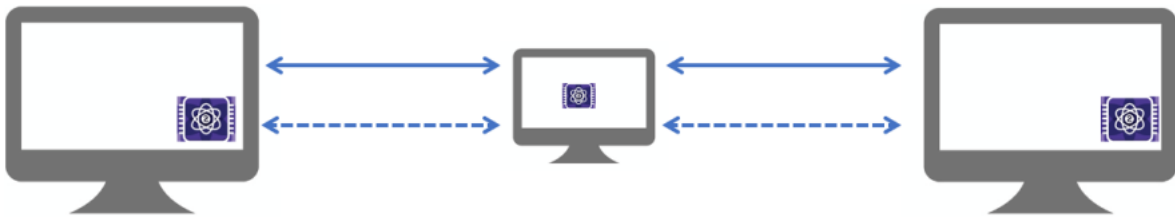
Figure 6.24 A quantum repeater separating the distance between Alice and Bob into segments, transferring the qubit from one segment to the other.
